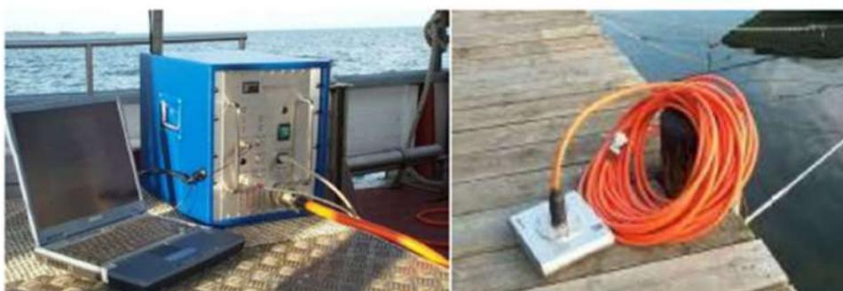
**Figura 15** - Sub-Bottom parametrico Innomar SES –2000 Compact.
